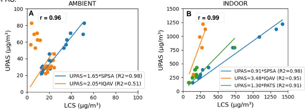
Fig. 3: Comparison between UPAS and low-cost sensors under ambient (A) and indoor (B) circumstances.
