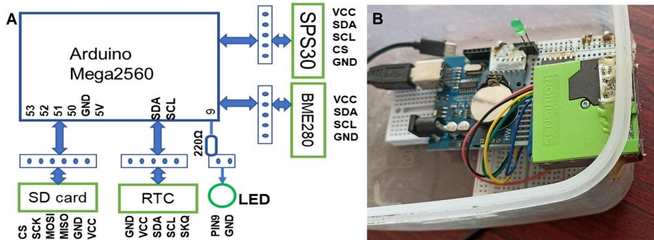
Fig. 1: Sketch of the SPSA circuit (A) and photo of the insides of an SPSA sensor system (B).
